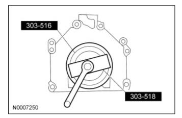
2. Using the Crankshaft Rear Oil Slinger Installer, install the crankshaft rear oil slinger.
