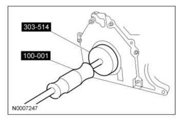
3. Using the Slide Hammer and the Crankshaft Rear Oil Seal Remover, remove the crankshaft rear seal.
